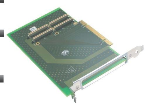
XS-PCI permits to use IEEE P1386.1 PCI Mezzanine Cards (PMC) in a standard PCI environment.
