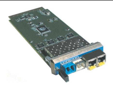
XS-AMC3 is an Advanced Mezzanine Card (AMC) which offers 10/100/1000 Ethernet connectivity in ATCA and uTCA systems.
