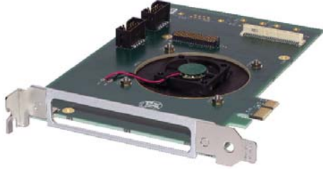
XS-PCIE2-100 (Low-profile fan, 3.6 CFM)
